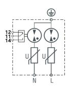
Surge protection 2-pole T2 with GDT and signal contact for IT/TT and TN network. Uc 385V.
